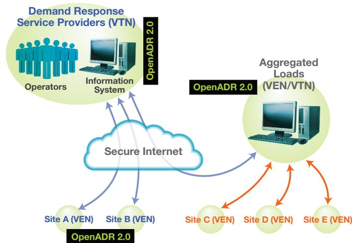
OpenADR’s Report Service initially targeted only storage resources and was used for battery telemetry to meet program requirements. The DRMS manages all aggregators of any resource as Vertical Top Nodes (VTN), as defined in the OpenADR architecture.
