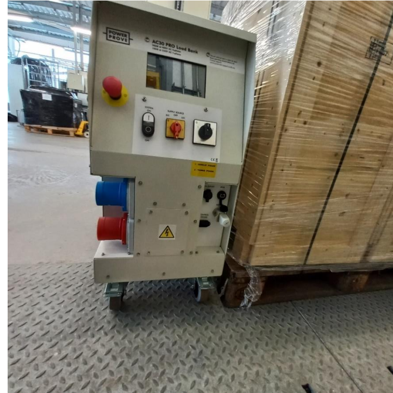
Controllable load bank for EV test rig
